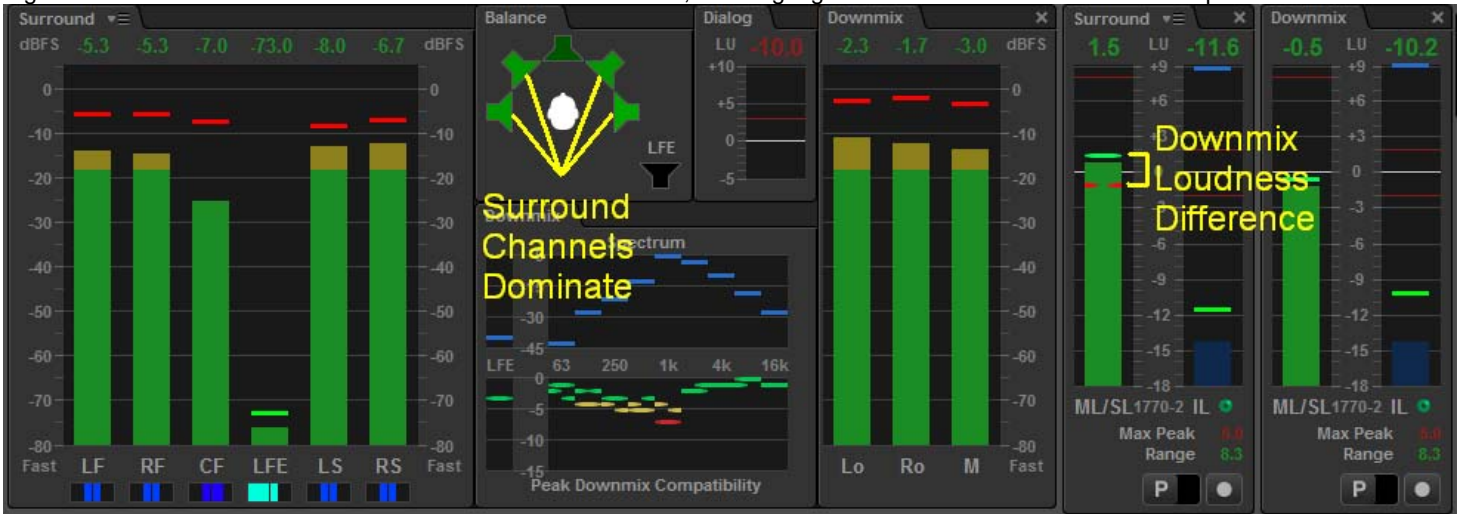
Figure 9b Measurements at cursor location “H” in timeline below, showing lower loudness when downmixed compared to surround
